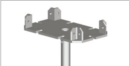
Bypass Head Used as an attachment to support two beams as stringers. Two beams can be supported side-by-side allowing for a continuous stringer line.
