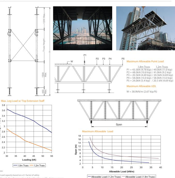
1) Load capacity based on a 2:1 factor of safety 2) Capacity for reference only and should not be used for design purposes.
